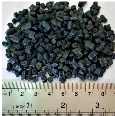
Fig. 3. Shape and dimensions of recycled nylon granules.
