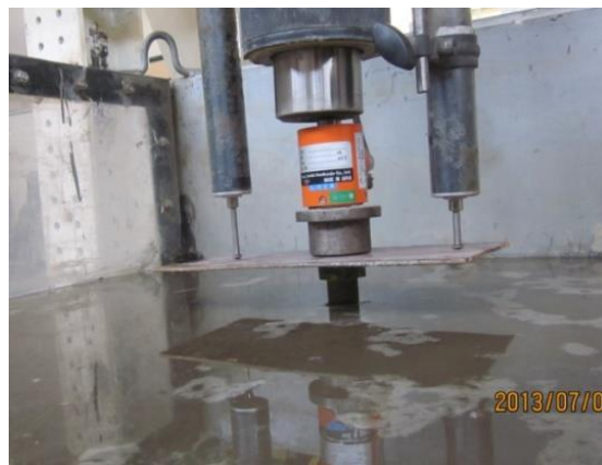
Fig. 3. Experimental setup for axial load testing.
