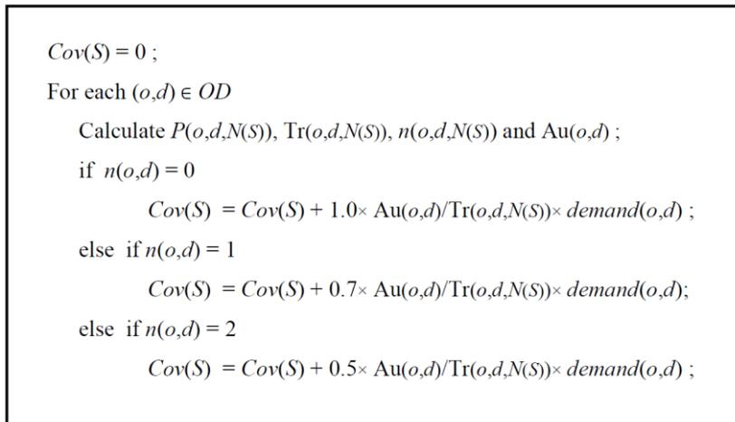
**Fig. 1. The process of calculating network coverage.**
