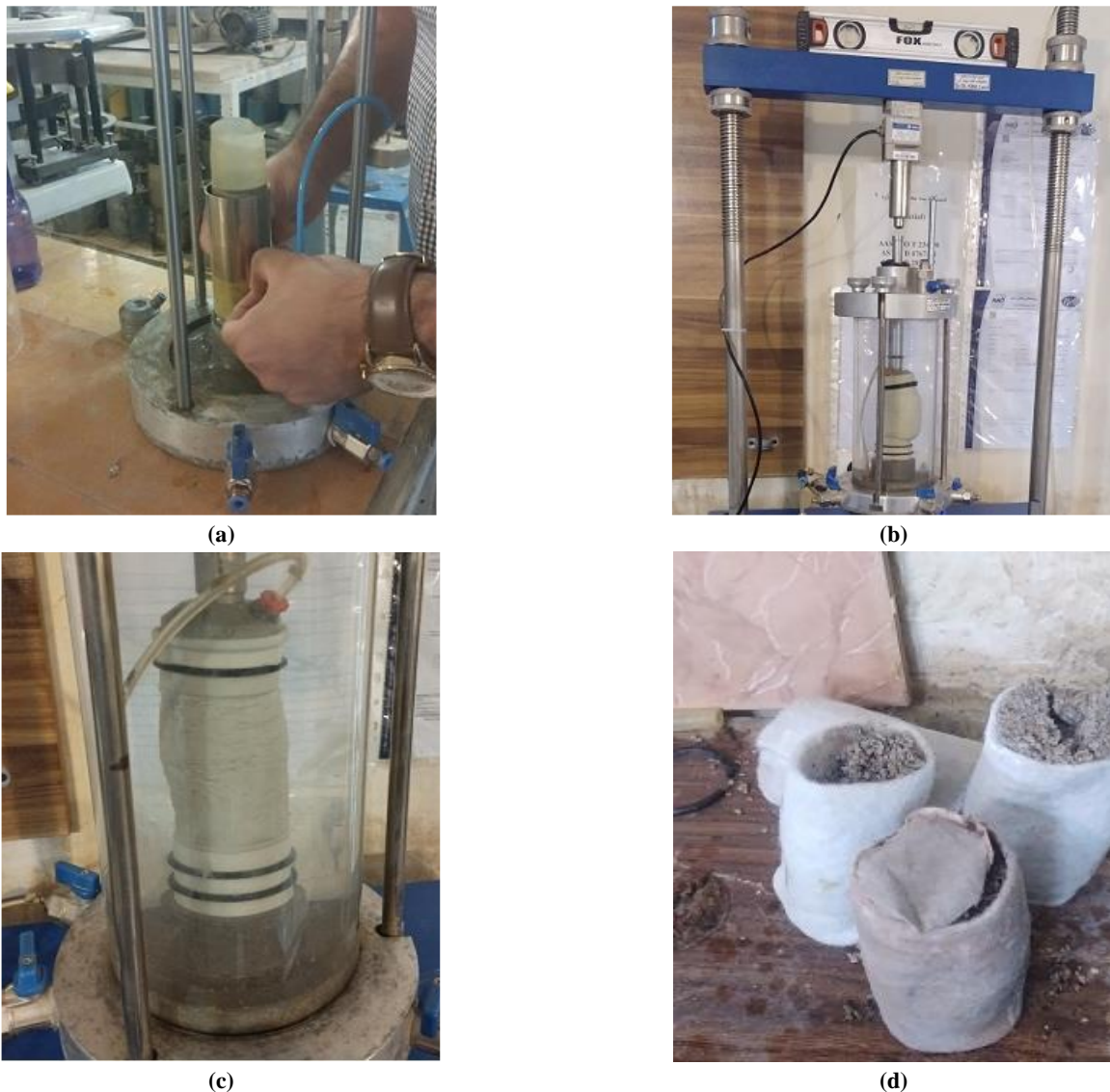
Fig. 4. Stages of the test execution: (a) Sample preparation, (b) and (c) Loading to failure, and (d) Geotextile-encased samples after failure.
