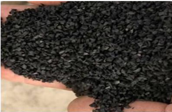
Fig. 3. Crumb rubber used in the samples.
