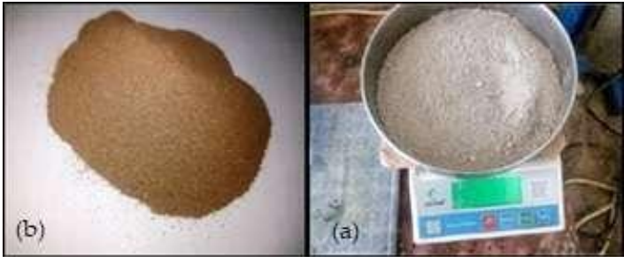
Fig. 2. Photographs of the (a) blast-furnace slag, and (b) ceramic powder used in the geopolymer concrete mixtures.
