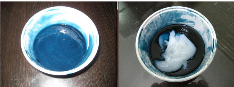
Fig. 4. Epoxy resin and hardener mixture.
