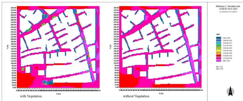
Map 3. Comparison of thermal comfort in the Laleh neighborhood in two cases without vegetation (right) and the current state (left)
