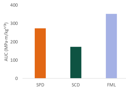
Fig. 21. Integrated performance index (area under \sigma_{max} – Z curve) for the three roof systems (SPD, SCD, FML). Lower values indicate better blast resistance.
