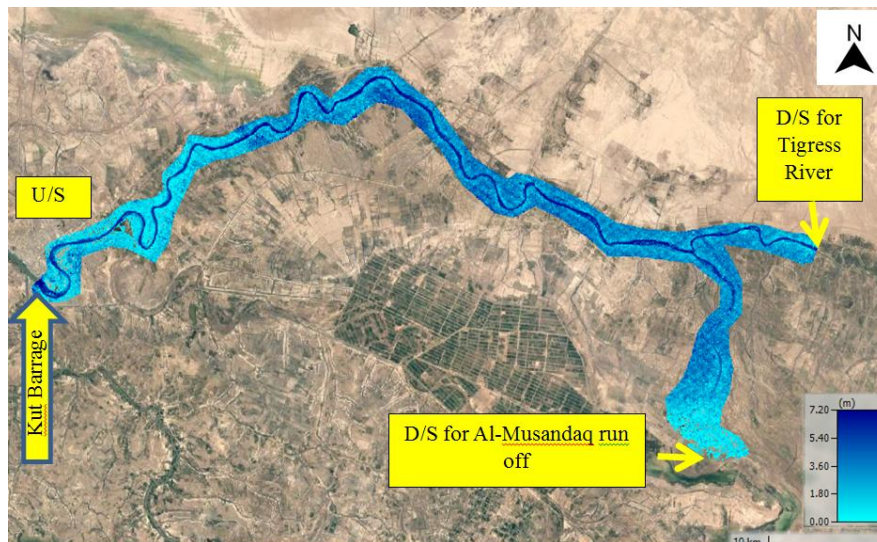
Fig. 6. Flow velocity field corresponding to the peak flow condition.
